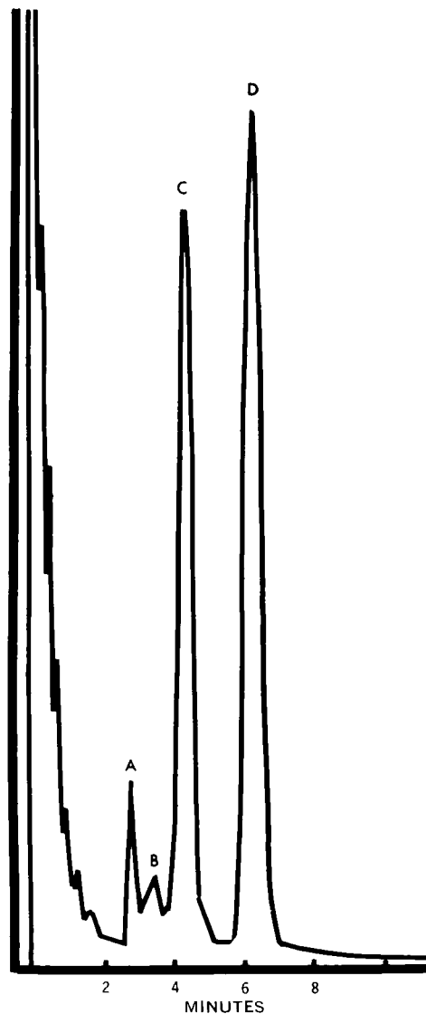
Figure 2 —GLC of derivatized ergonovine maleate (for conditions see text). Key: Peak A, derivatized ergonovine; Peak B, derivatized lumiergonovine I; Peak C, derivatized ergonovine; and Peak D, brucine (internal standard).
